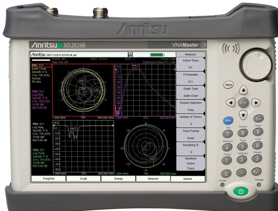
VNA Master™ MS202xB/MS203xB Vector Network Analyzer + Spectrum Analyzer Compact Size: 199 mm x 273 mm x 91 mm (7.8 in x 10.7 in x 3.6 in), Lightweight: 3.5 kg (7.6 lb)
